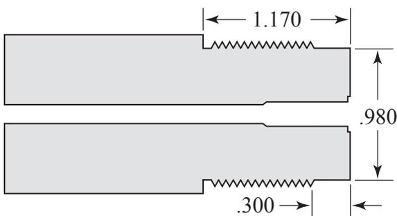
When chambering cut tenon 1.0600" in diameter by 1.170" long, except cut last .300" at .980" diameter.
