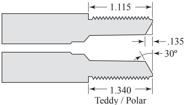
When chambering cut tenon 1.0600" in diameter by 1.115" long for a Panda, Short Kodiak or Grizzly II, .980" long for a Long Big Bore Panda, Long Kodiak or Long Grizzly II, .692" long for Cone Bolt Atlas, .557" long for Flat Bolt or Long Atlas, or 1.340" long for a Teddy or Polar. Leave rear end of barrel square for now.
