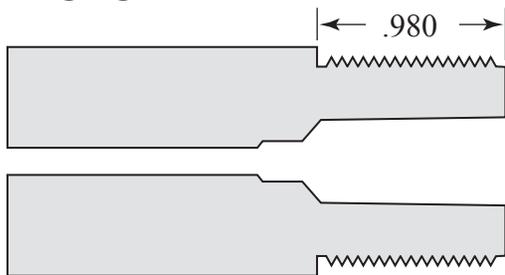
For a coned bolt run the chambering reamer in until head-space gauge is flush with rear end of barrel. For a flat bolt run the chambering reamer in until measurement from base of head-space gauge to shoulder of barrel is 1.115".
